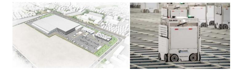
The CFC is characterized by its ability to hold a large range of approximately 50,000 products. It is enabled by 24 hours, highly efficient picking operations using robotics and AI. By utilizing Ocado's solution, the robots in the CFC can assemble a 50-item order within 6 minutes. Advanced AI algorithms are also used to constantly identify and update optimal routes for the most efficient home delivery.
