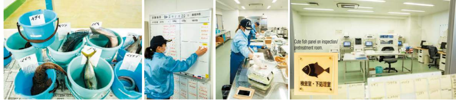
Far left: All species of fish caught that day are tested for radioactive substances. Middle left: The process is managed on a whiteboard to make sure all fish types are tested. Middle right: Fish are filleted or minced for testing. Far right: The inspection room has 9 devices to measure the level of radioactive materials.
